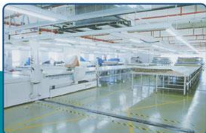
Supporting air bed scene in real use of automated cutting machine
